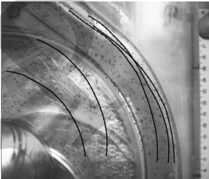
图 6 试验所得模型泵内颗粒运动轨迹 Fig. 6 Particle trajectories in model pump obtained by experiment
